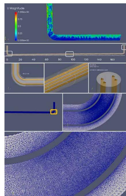
Both the third-party and open-source simulation packages have been ported to a Cloud-based HPC system. The resultant simulations have enabled Prysmian to improve the calculation of losses inside an energy cable, especially those induced by the magnetic field from the load current. They are also able to model better the heat transfer from the cable to the surrounding environment.
