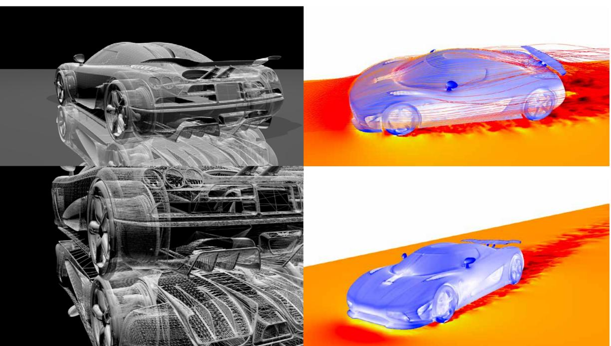
The challenge facing Koenigsegg was to perform simulations of the flow over its hypercars which were sufficiently detailed to model real physical effects accurately.
