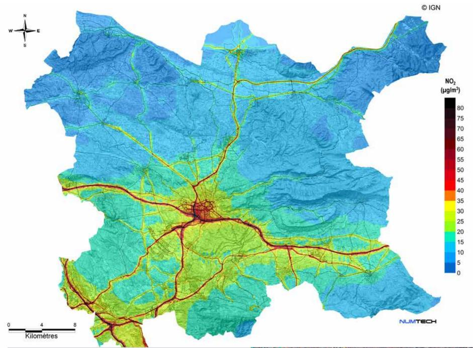
The challenge of this case study was to demonstrate the use of Cloud-based-HPC services to investigate air-quality at the scale of cities. This case study used the ADMS-Urban software from CERC running on the Extreme Factory HPC offering from BULL.
